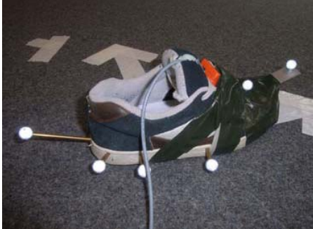
Figure 2. Photograph of shoe #1 showing the IR reflectors tracked by the optical tracking system. The IMU is firmly attached at the instep of the shoe
