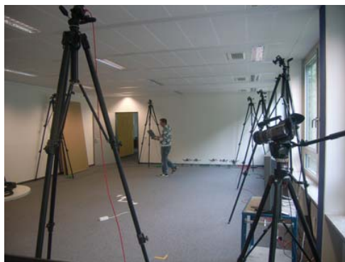
Figure 1. Photograph of the optical tracking system. The camera on the right was used to make a video recording of each experiment
