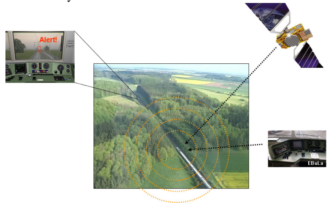
Fig. 1. Principle of collision avoidance based on the broadcast of traffic relevant information among vehicles, illustrated for the railway case.
