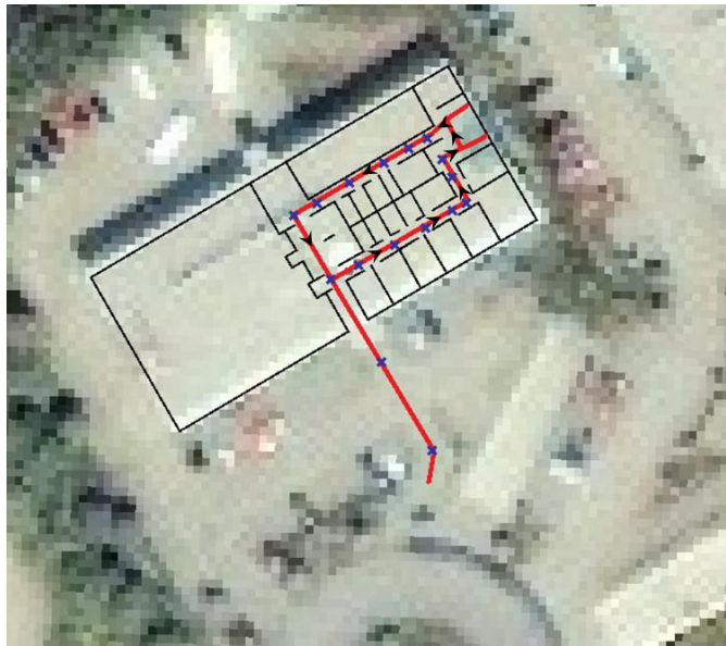
Fig. 4. An evaluation scenario, where the red line shows the path followed by the test user. The ground truth points are visualized using the blue crosses.
